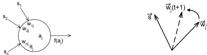
Fig. 3. McCulloch-Pitts Neuron (left), Adjustment of a weight vector to an input pattern (right)
