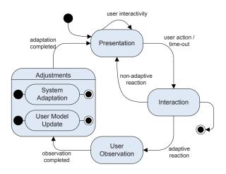
Figure 7: Lifecycle Model of Adaptation (Munich Model)
