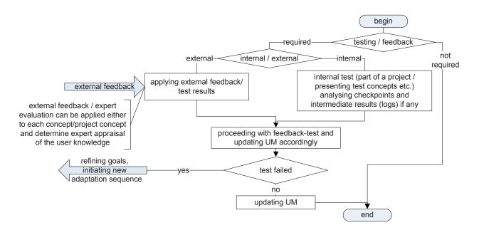
Figure 12: Test-feedback functionality flowchart
